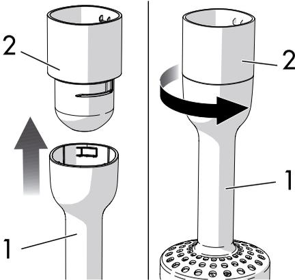
3. Then proceed to attach the potato masher and gearbox unit to the hand blender body (3).
