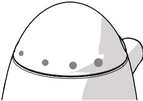
It allows you to adjust the blades' rotation speed while using the hand blender. The speed adjustment is progressive: the dots on the selector become larger to indicate a speed increase.
